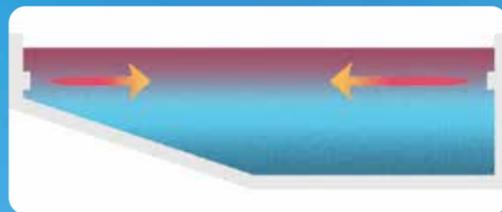
Standard circulation systems only move water at the surface, creating cold spots, layering and poor sanitisation.
