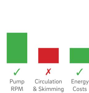
Variable speed pumps are appealing because they present an opportunity to reduce energy costs. Whilst they can turn over a sufficient volume of water at lower pump speeds, skimming power and circulation is compromised. Without sufficient skimming and circulation, water balance is difficult to maintain, algae forms in dead spots and maintenance costs increase significantly.
