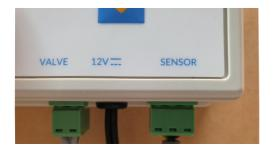
NOTE: Sensor and Solenoid plugs must face backwards when inserted into the new Water Witch Control Box.
