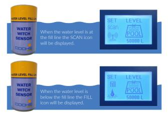
If you do not press **ENTER** to confirm the sensor level the unit will remain in **SET LEVEL MODE**.
